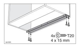
Screw the spacer strip underneath the housing unit sides, flush with the rear wall.
